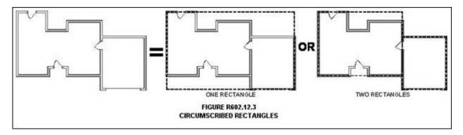
**R602.12.4 Required length of bracing.** The required length of bracing for each side of a circumscribed rectangle shall be determined using Table R602.12.4. Where multiple rectangles share a common side or sides, the required length of bracing shall equal the sum of the required lengths from all shared rectangle sides.
