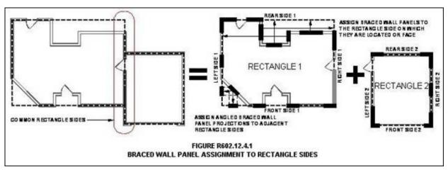
3. The projections of angled braced wall panels shall be assigned to the adjacent rectangle sides.
