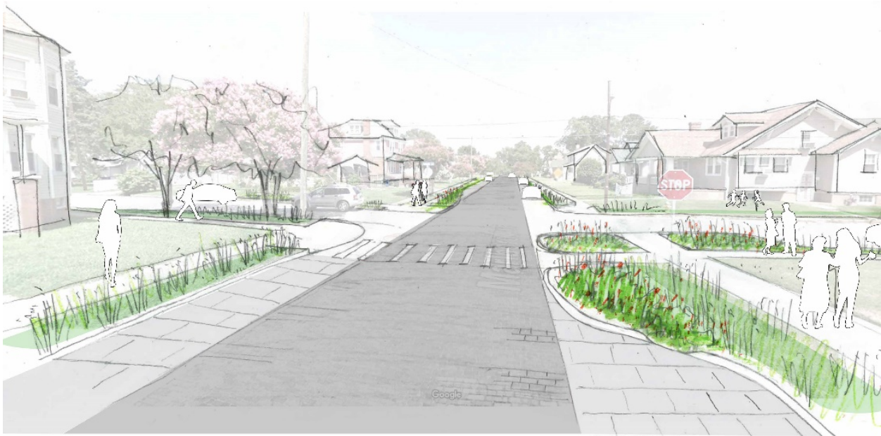
Rendering of permeable pavers along the sides of the street at the locations of on street parking. Source: SCAPE.
