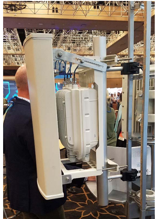
CBRS 3.65GHz Sector and Base Station Display
