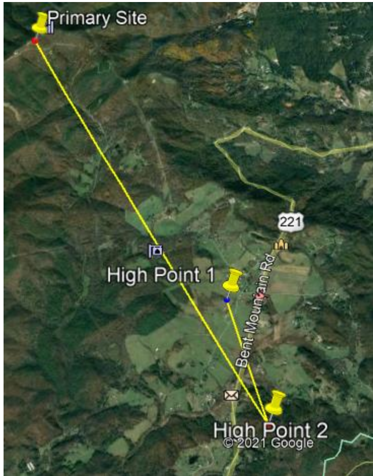
Image – Backhaul Connections between sites
